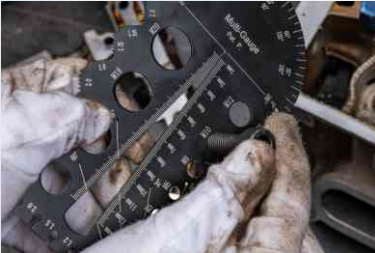
Gage Holes Measure the Major Diameter of Bolt
