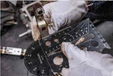
Gage Leg Quick-Check Perpendicularity
