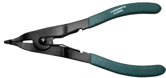
JOA720 A1040005 Lock Ring Pliers (Angle Tip) Removing and installing all types of lock rings. Used in brakes, transmission, pedal shafts, clutches shaft. Deep serration jaws hold lock rings securely
