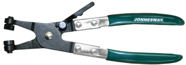
JOA607 AR060003 Swivel Jaw Hose Clamp Pliers "V" slot For easy removal & installation of ring type hose clamps. Jaws swivel to grip any angle
