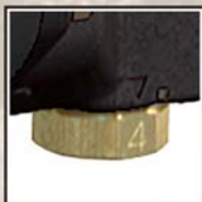
Air Regulator 4 torque setting.
