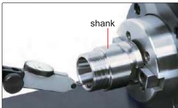
measure radial runout of shank
