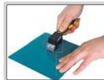
step 1: make grid cutting on surface
