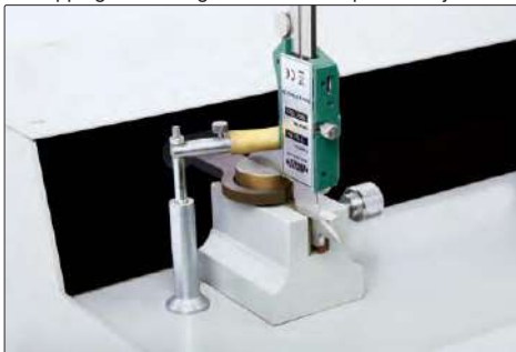
lapping measuring surfaces of caliper lower jaws
