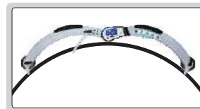
external diameter measurement
