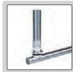
test cylinder surfaces (use V-groove on the cover)
