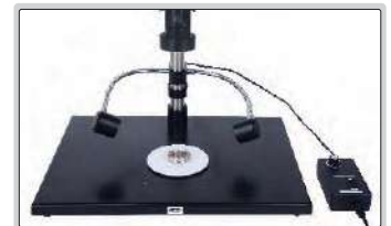
illumination direction and brightness are adjustable
