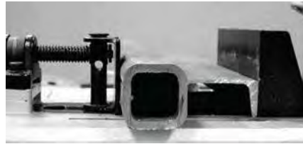
Square & Rectangle Tubing (use block spacer)
