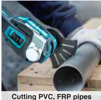
Cutting PVC, FRP pipes
