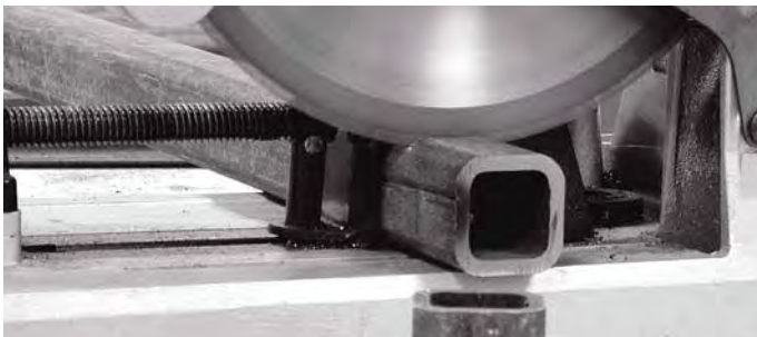
Carbide-Tipped Blades make Virtually Spark-Free Cuts
